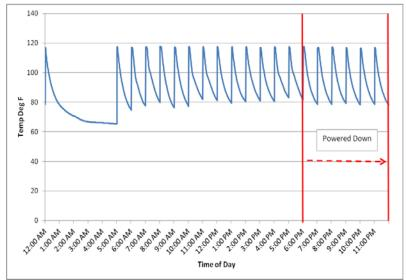
But the addition of one more hour to the shutdown caused the unitary system to deliver colder water in the last draw of the day, as shown in Figure 8 (Sullivan et al., p. 3.8). The split system with its 80-gallon tank provided setpoint hot water after being shut down for 12 hours.
