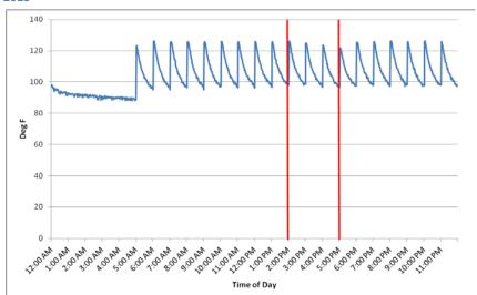
Figure 14. ERWH Oversupply Delivered Water Temperature Profile: 2:00 p.m. to 5:00 p.m. Powered-down Protocol, June 13, 2013
