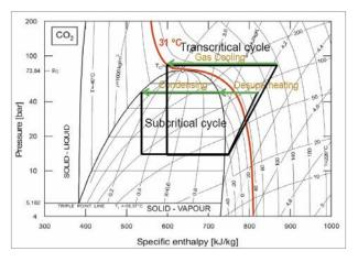
state from a liquid/vapor mixture to a gas. The compressor then lifts the  $CO_2$  back to the transcritical zone where it transfers heat to the colder water.
