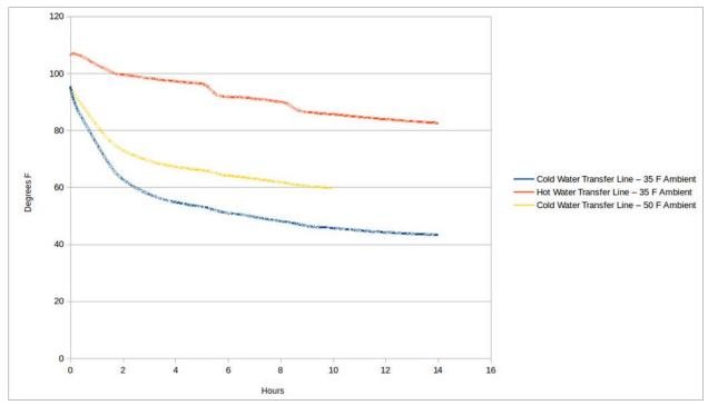
Figure 24. GAU Split-System Water Transfer Line Temperature Profile
