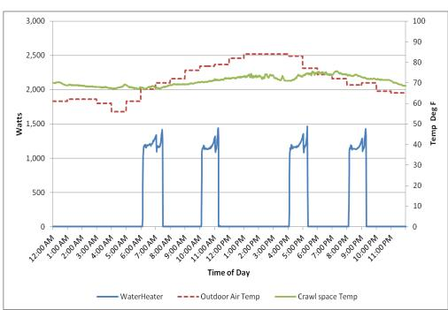
Figure 5. Compressor On and Energy Consumed: 40-gallon Unitary System
