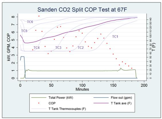
Figure 17. COP Test at 67°F Ambient – Split System
