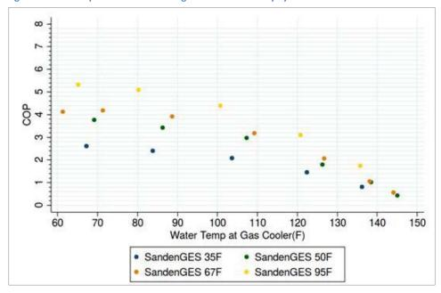
Figure 18. COP Map for Sanden GES 40-gallon Tank – Unitary System
