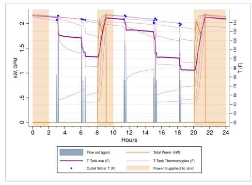
The split system operated only once during the midday ON period at 35°F, but operated at the start of the midday and midnight power-on periods at 50°F and only at midnight during the 67.5°F test. Like the unitary system, the split system used less electricity and lower power capacity as the supply air temperature increased. In the Ecotope report, graphs for both systems at all temperatures are shown. **Figure 23** shows the split system operation.
